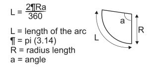
A sheet metal worker has to design a cone which has a circular base. The radius (R) is 5 metres and the angle (a) is 30°. What will be the diameter of the base of the cone? (You also need to know the formula for the circumference of a circle.)
