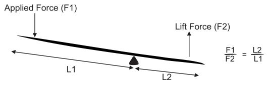
1. A 100 kg weight is applied to one end of a leaver 2.2 metres long. The leaver is pivoted 0.2 metres from its end. What lift force is exerted?
